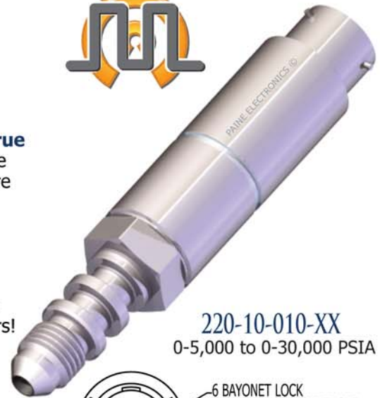
6 BAYONET LOCK ELECTRICAL RECEPTACLE MATES WITH MS3116-10-6S
